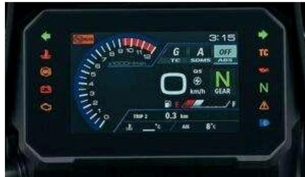
The display now adds a function to display pop-up large alerts and warnings. The tachometer also serves as a programmable engine rpm indicator. It blinks when the engine speed reaches the preset rpm entered by the rider. It can be set in 250rpm increments within a range from 4000rpm to 9250rpm.
