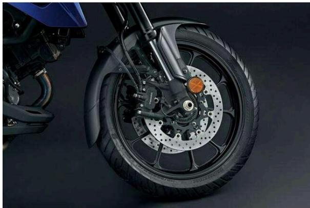
Four-piston front caliper
