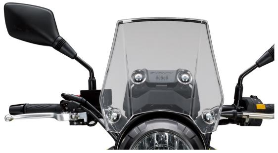
While compact, the windscreen benefits from repeated wind tunnel testing to optimize its shape, providing highly effective shielding for a more comfortable ride.
