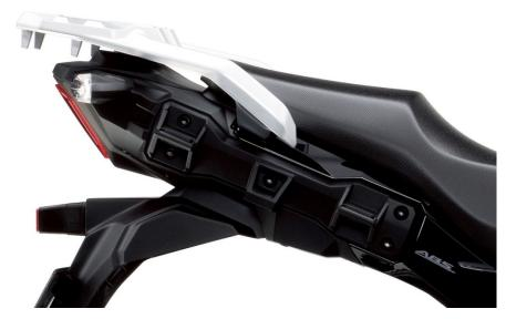
Designing dedicated mounting clips to accommodate the optional side cases makes realizes an integrated design that matches the bike. The large aluminum rear carrier with 8.5kg maximum capacity is fitted with hooks for attaching straps and that can also be used for attaching the optional top case.
